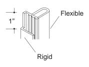
Install the vinyl extrusions on the right and left side of the apron.
